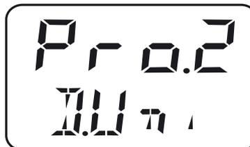
Pro.2 = the measured value is displayed as a percentage of the scaled measuring range, See section 7.8.1 "Setting the starting value of scaling (Sc.Lo)", page 35 and See section 7.8.2 "Setting the final value of scaling (Sc.Hi)", page 36.
